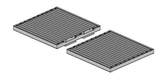
Note: If no reticulating ductwork is above the slab a protective and load-bearing grate is necessary.
