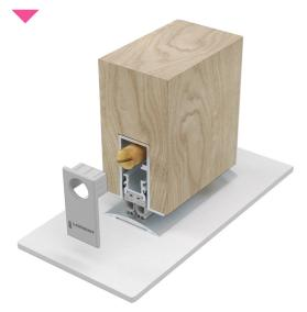
LAS8012 si & LAS8013 si are heavy-duty aluminium drop seals featuring twin gaskets for excellent acoustic performance. Both seals feature a high efficiency mechanism, which lift the seals clear of the floor as soon as the door is opened by a few millimetres. They require no power connection.
